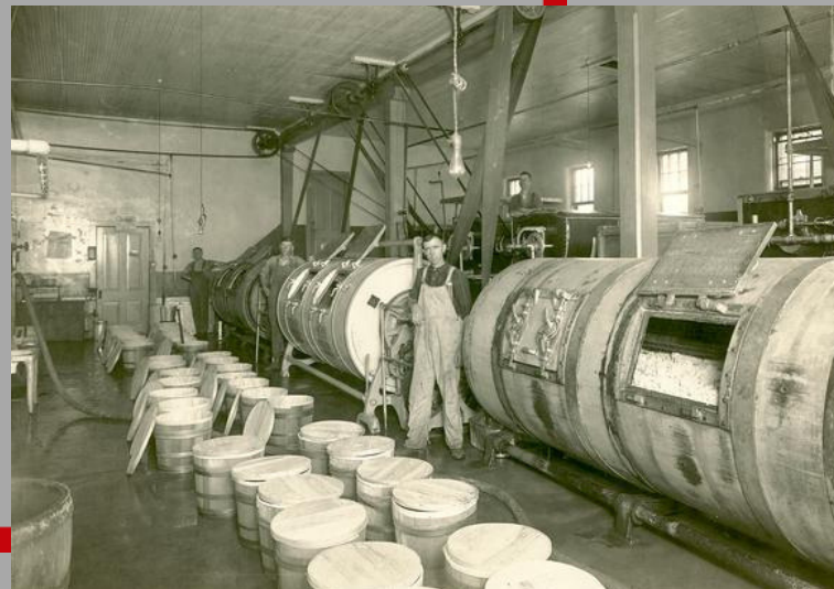
Two men pose at the Barron Coop Creamery (Dairy) next to the churns full of butter, which is ready to be packed into the small barrels nearby. Barron, WI, USA.c. 1900, WHS #3238
